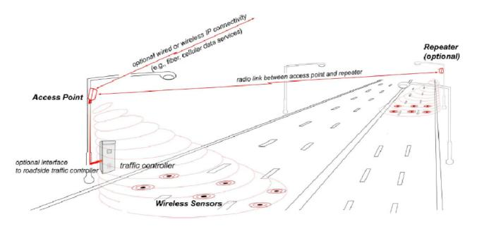
The Access Points are usually mounted on top of a suitably positioned signal head. The Repeater Units, where needed, are battery powered, with either two or seven year replaceable battery options available. Each repeater can support up to 10 sensors, also within a 30m range, relaying the detection data back to Access Point and extends the range of an Access Point by up to 300m.
